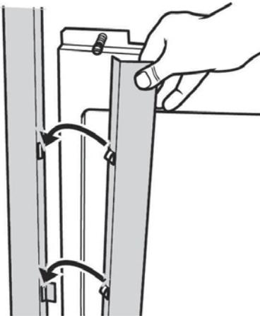
4. Fit the barrier screen hooking its bottom tabs to the bottom of the side channels and snapping its top tabs to the top of the side channels.
