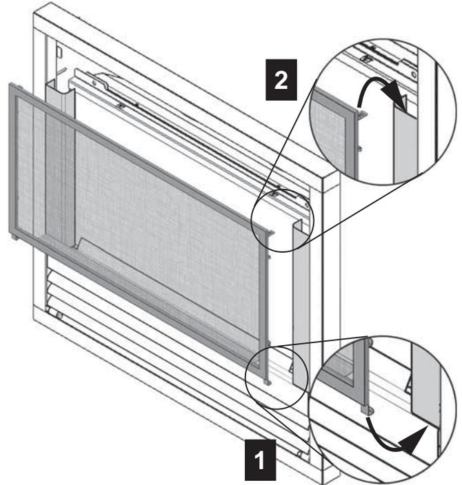
5. Slide the lower edge of the upper louver behind the screen and attach the louver by hooking it over the tabs near the top of the firebox sides.
