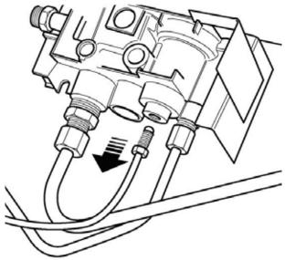
5. Fit the thermocouple interrupter block to the valve. Do not overtighten. Finger tighten approximatively 1/4 of a turn.
