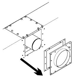
2. Fit the rear cover plate (supplied with the kit) using the seal and 12 screws previously removed. The hole in the cover plate must be nearest the top edge.
