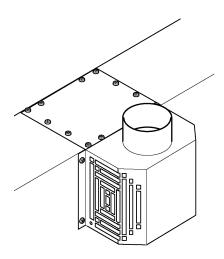
4. Fit a "P" clip at the bottom rear right corner of the appliance case. Fit the vent switch wire to the clip. Feed the wire into the case through the hole at the bottom corner.
