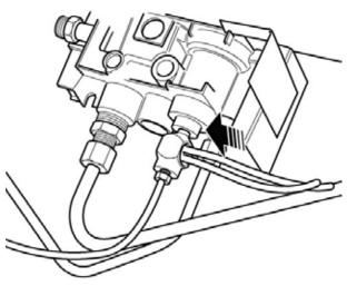
7. If the appliance is to be fixed to the floor, don't attach the burner module to the appliance yet. Wait until the appliance is accurately positioned with the B-vent attached. The holes in the appliance base for floor fixing are not accessible when the burner module is fitted.
