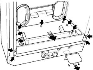
3. Fit a "P" clip at the right side of the inside of the case. Fit the vent switch wire to the clip.
