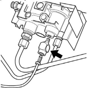
6. Connect the vent switch wires into the thermocouple interrupter block. Screw the thermocouple into the interrupter block until finger tight. Make sure that the wires are properly located and finally tighten the thermocouple nut (approx. 1/4 turn) with a wrench to secure the wires with good contact.
