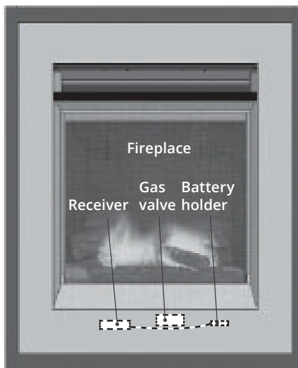
Battery holder located next to gas valve on bottom of fireplace behind access panel/fret
