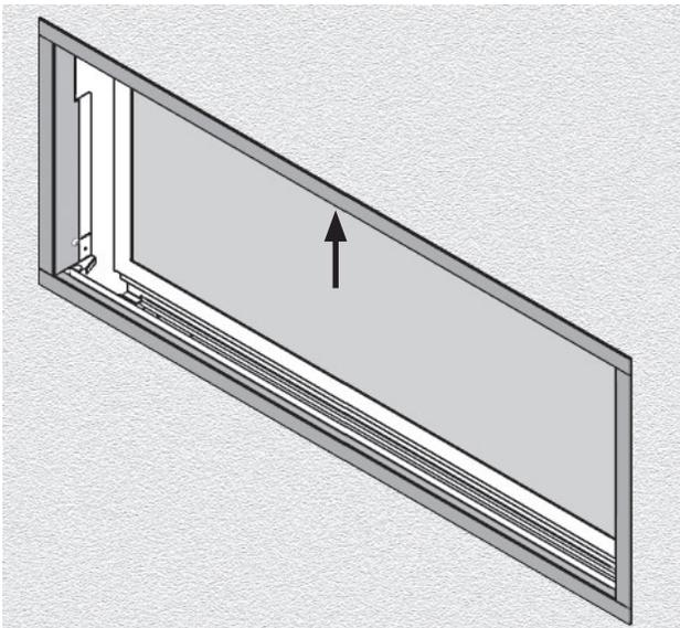
4. Place the plinth in the space between the glass and the trim. Align the round notch of the plinth to the hole in support underneath as shown.
