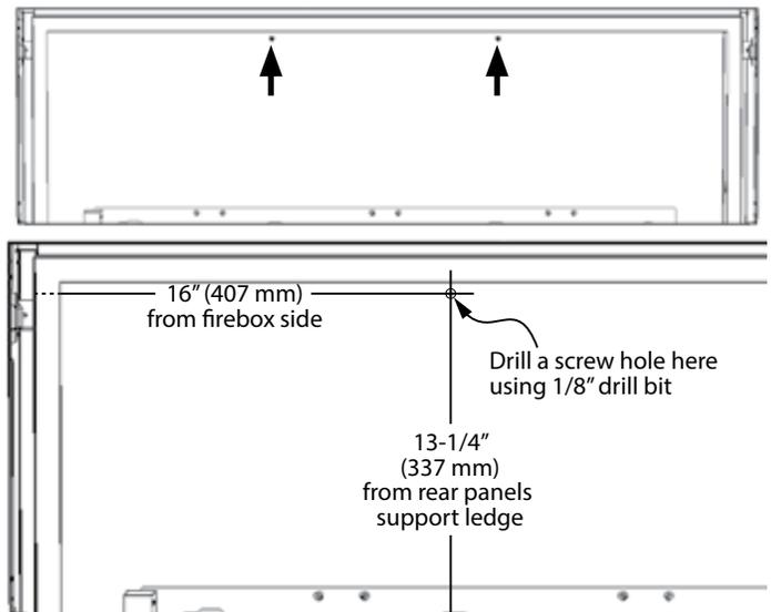
holes for the glass panels anchors as indicated, using 1/8" drill bit. Use the measurements indicated below and repeat on both sides.
