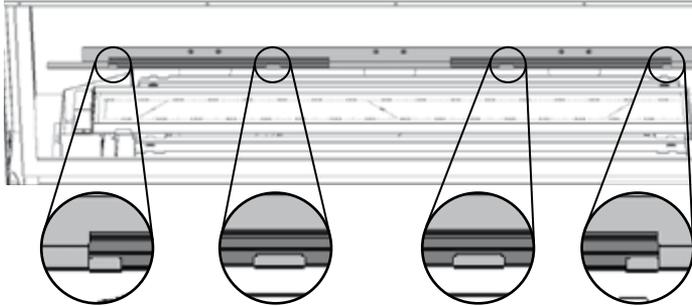
back, on the ledge of the firebox behind the burner. The strip are held in place with the tabs of the ledge as indicated below.
