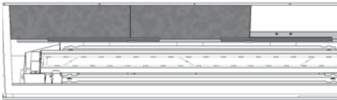
of the retainer strip. The left panel will overhang the strip on the left. The right panel will overhang the strip on the right. The middle panel straddle both strips.
