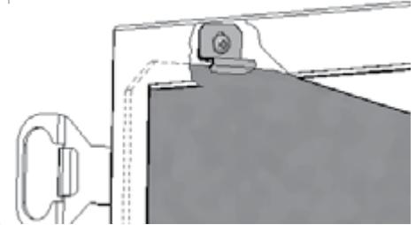
When installed, the top panel rests at the rear and sides on the glass panels and their anchors. In the front, it rests on the top panel support bracket inside the front edge of the firebox. Position and slide the top panel into the left corner of the firebox.
