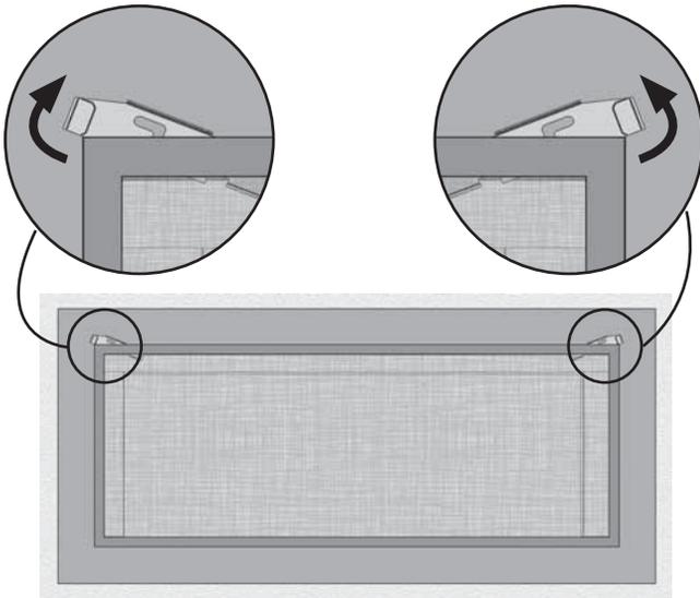
4. While holding the screen, rotate the lock-in levers so that they hook onto the trim, then slide the levers inwards to secure the screen to the trim as indicated.
