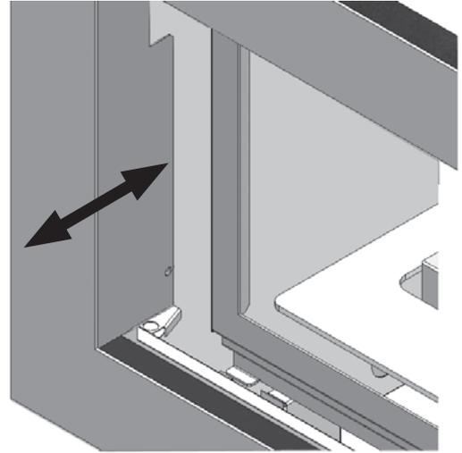
2. Select a pre punched hole and secure trim using 4 no 8 screws.
