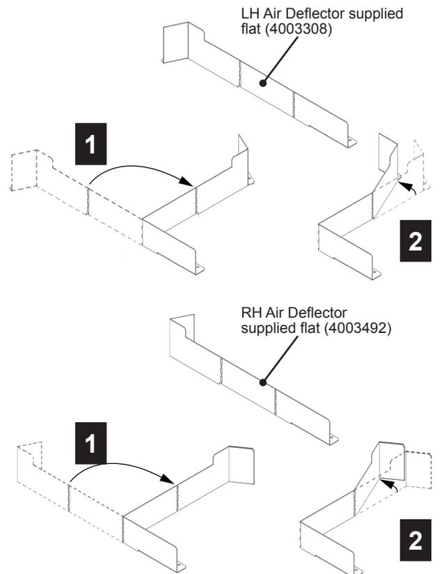
4. Install the air deflectors as shown. Fix them in place with 3 existing screws already in the firebox as indicated.
