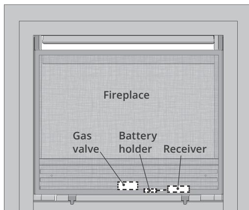
Battery holder located next to receiver on bottom of fireplace behind access panel/fret
