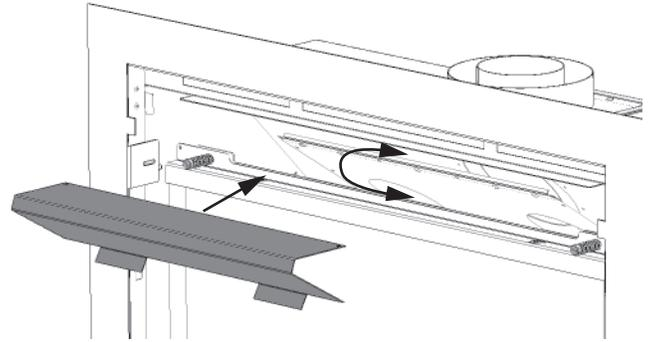
4. Place the access panel horizontally under the screen and insert the pins on each side of the frame through the slots in the panel. Rotate the panel downward.
