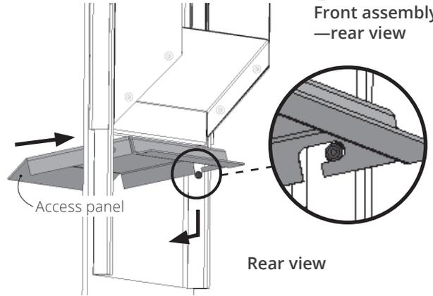
5. Hook the Front Assembly to the four tabs inside the backing plate.
