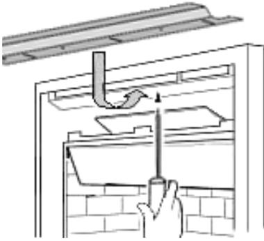
3. Place the heat exchanger cover over the heat exchanger. Note its shape and orientation.
