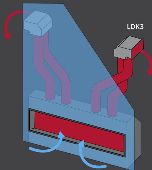
HeatShift naturally delivers up to 125 cubic feet of hot air per minute—without a fan!
