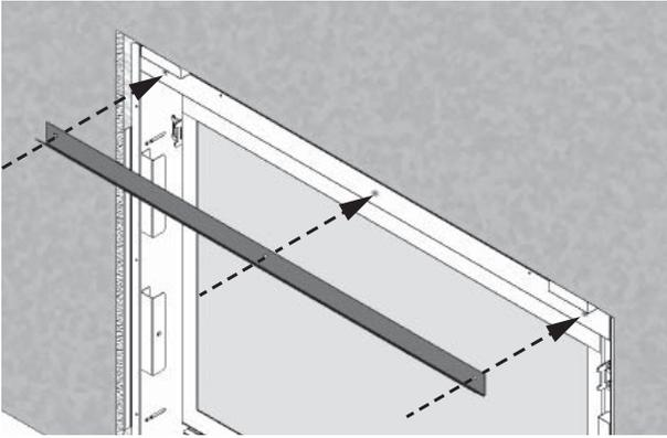
2. Install the door catch bracket to the bottom of the backing plate (2 screws). You can add some washers (supplied) to shim the door catch if it is too low and the door is too easy to open.
