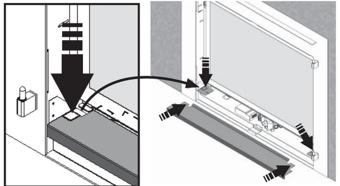
5. Adjust the position of the convection brackets on each side of the window. Release the nut, pull the bracket as far forward as possible and tighten the nut.
