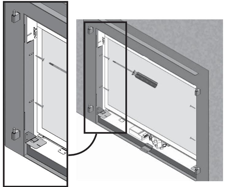
4. Slide the removable panel in the clip on the horizontal supports on each side and push it in until flush with the backing plate.
