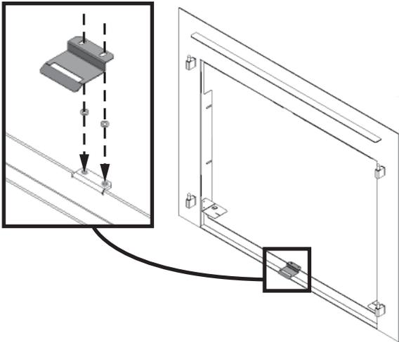
3. Carefully position and secure backing plate with 4 low profile screws to 4 firebox mounting brackets. Before tightening, push the plate against the wall finish then tighten.
