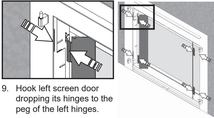
9. Hook left screen door dropping its hinges to the peg of the left hinges.
