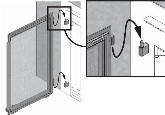
11. Close first the left door pushing on it firmly so that the tab at the bottom of the door snaps into the door catch. Close the right door. If the doors are too easy to open, add some washers underneath the door catch to raise it—see step 2.
