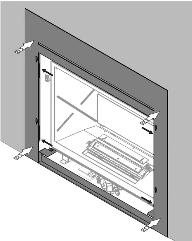
2. Slide the removable panel into the clips in the side panels.
