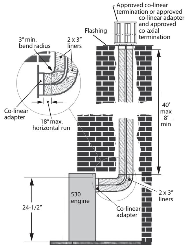
**Vertical co-linear installation into existing F/P**
