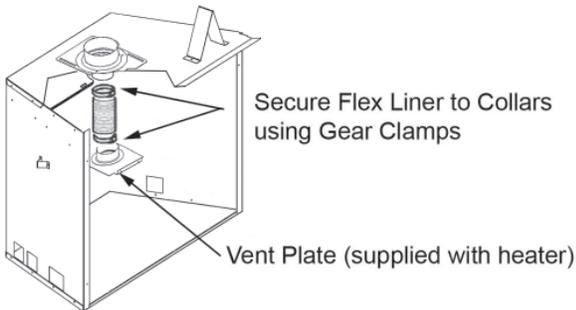
5. Compress or stretch the liner so the vent plate is approximately 19" above the floor.
