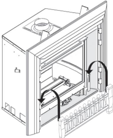
Hook fret onto fret retainer brackets (RA24FK) using RA24DS style front
