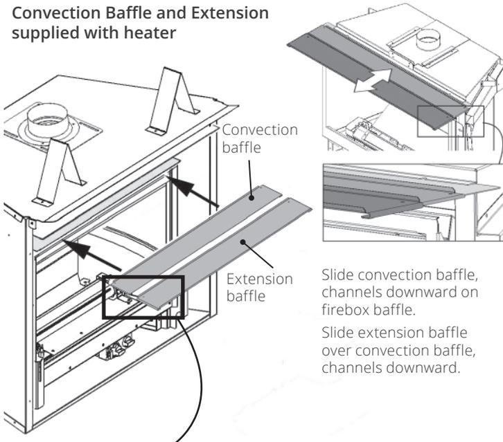
Slide convection baffle, channels downward on firebox baffle.
