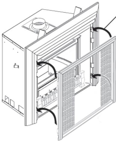
Hook inner front trim onto mounting brackets within outer trim.
