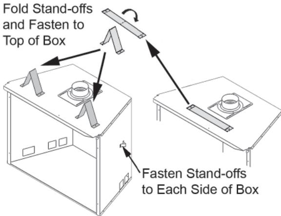
2. Position ZC box in cavity and connect to vent system—see note above concerning the position of the ZC box.
