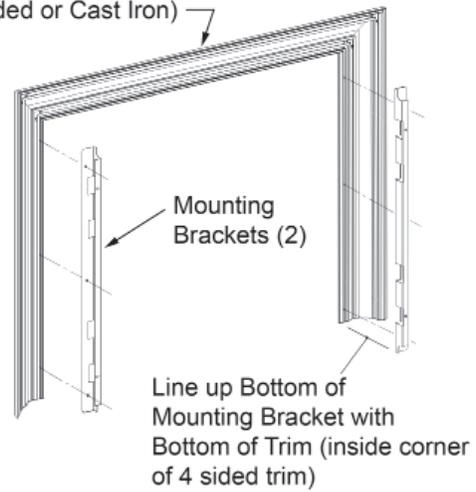
Note: It may be necessary to extend the outer trim to cover the combustible wall opening. Custom non-combustible sheet metal pieces may be added to the extruded aluminum trims and fastened using the screw channel on the back of the trim.
