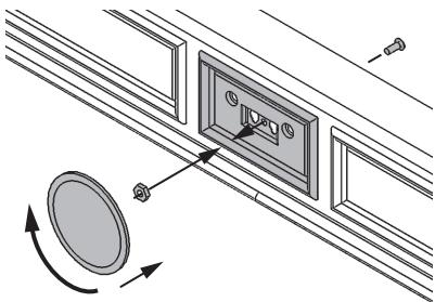
4. Install the cast surround fitted with mounting brackets to the heater using 4 screws provided.
