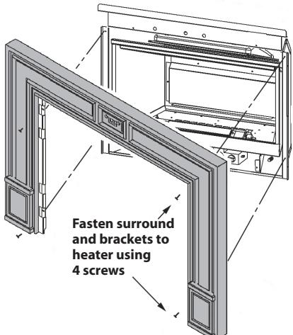
**NOTE:** Where further fixing is required, fasten the surround to wall using screws through 2 outermost holes at the top centre of the surround. Backing or wall anchors (not supplied) may be required for fastening.
