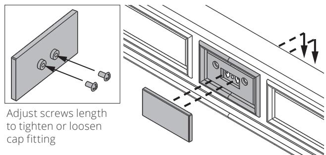
6. Clip the selected trim (supplied separately) onto the mounting brackets within the cast surround.
