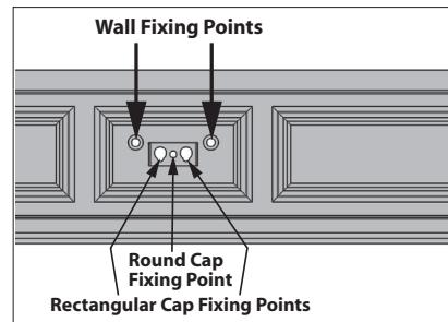
5. The rectangular cap can be fitted to the surround after the surround is installed. Simply fit the screws provided to the back of the cap and hook the cap to the surround through the 2 keyholes at the top center.
