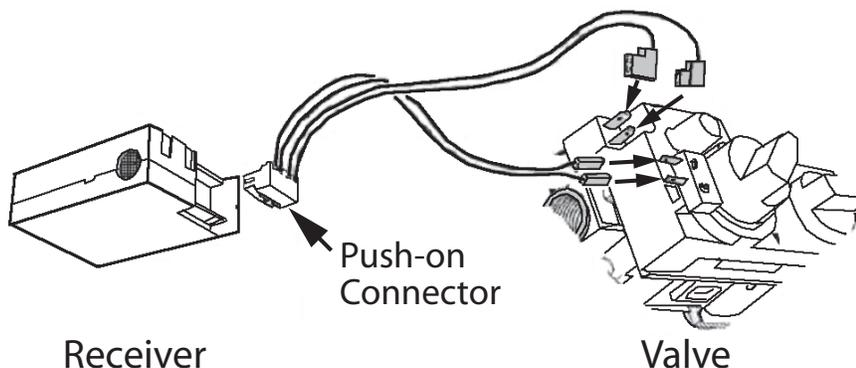
**CAUTION! Don't put the batteries in the remote control receiver until the wires are connected to the gas valve, as short circuit could result in destruction of the electrical components.**
